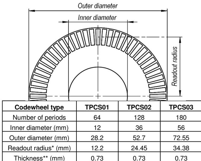
\* Readout Radius = position of encoder center
